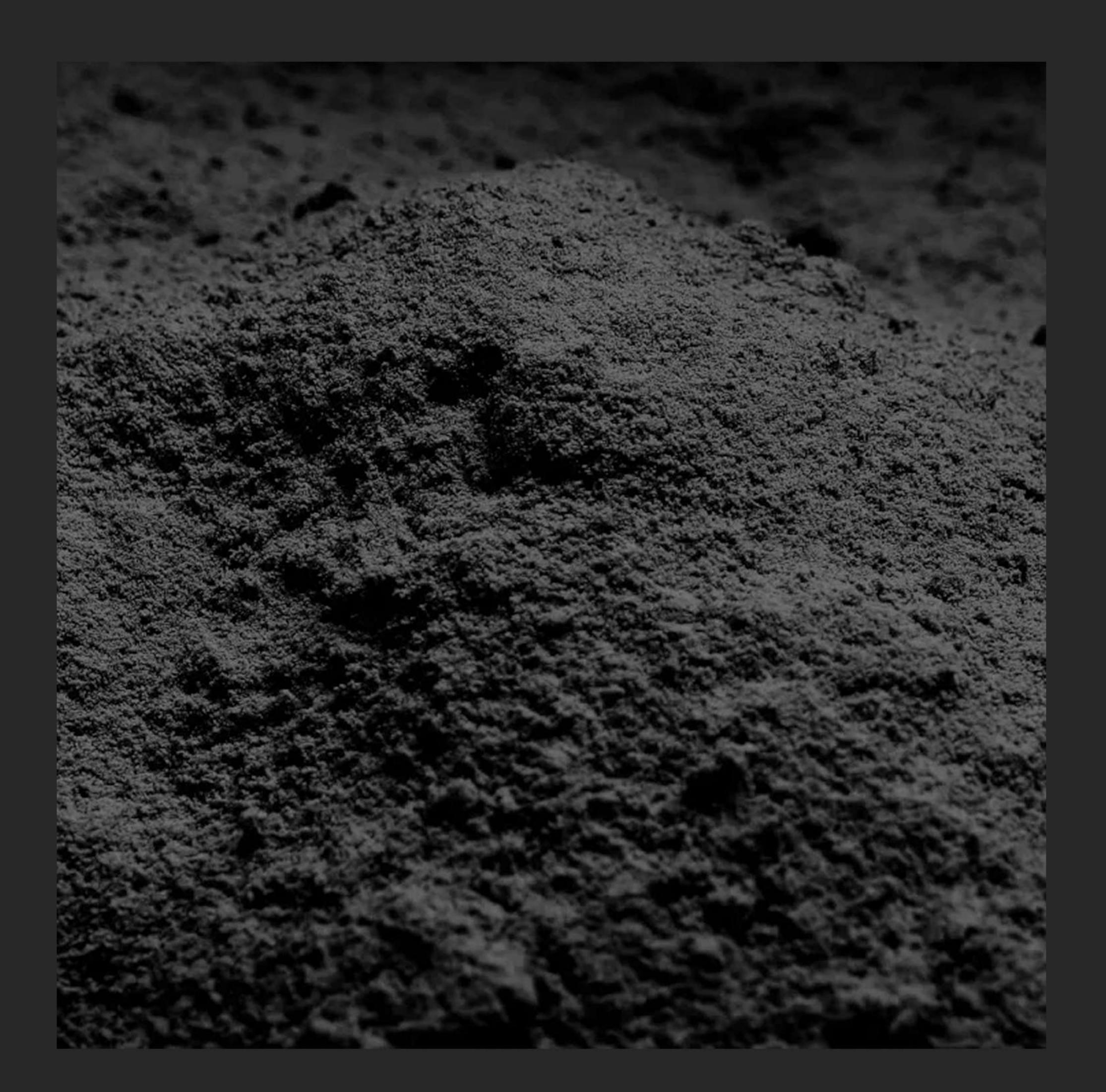
Carbon black is virtually pure elemental carbon in the form of colloidal particles that are produced by incomplete combustion or thermal decomposition of gaseous or liquid hydrocarbons under controlled conditions and is composed of fine particles consisting mainly of carbon.
